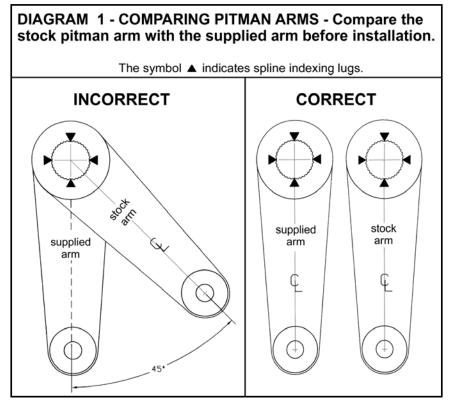
after 3/1/99) on the sector shaft in the exact same position as the original arm. Reinstall the factory jam nut and tighten (200)
