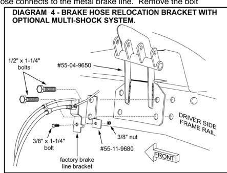
□□ Carefully bend the hard line down from the factory position and attach the factory bracket to the "10" and "11" bracket as shown using the supplied 3/8" x 1-1/4" bolt and nyloc nut (33).
