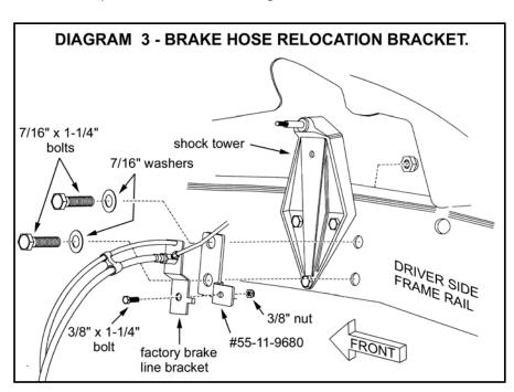
□□ [DIAGRAM 3] Install the brake line relocation bracket (#55-11-9680 driver side and #55-10-9680 passenger side) below its factory position using two existing holes in the frame as indicated. Secure this bracket using the supplied 7/16" x 1-1/4" bolts, flat washers, and nyloc nuts (52). The washers should be installed under the bolt heads.
