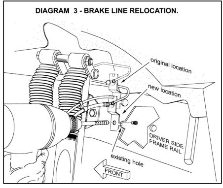
**WARNING:** Use extreme caution when bending the brake hard line. Avoid pinching or crimping the line, and adjust the line as necessary to avoid contact with any other components.
