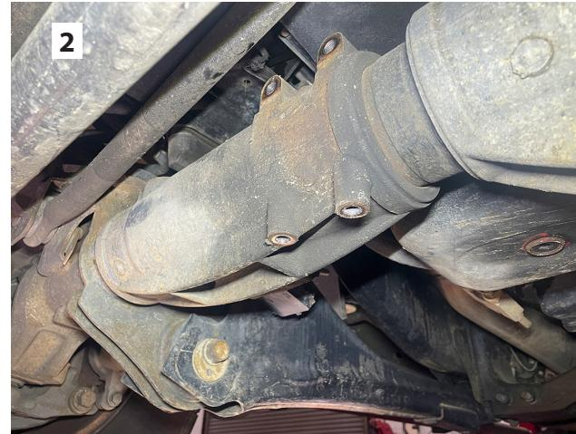
4. [Illustration 3] Remove the factory steering stabilizer mounting bracket from the tie rod.
