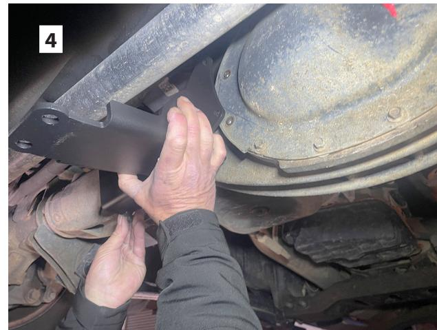
8. [Illustration 5] Place the new differential spacer (55-06-92770) between the center bracket assembly and the differential and secure using supplied 8mm bolts and washers, applying the supplied thread locker to the bolts.
